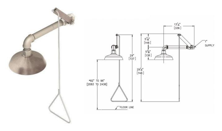
Model S2200-AS is our horizontal wall mounted safety shower with stainless steel head. Supplied with stainless steel pull handle and 1" stainless steel stay open ball valve and stainless steel pipework.
